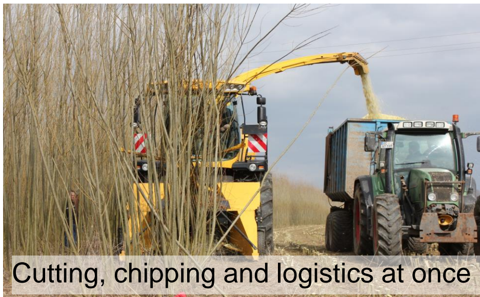
Figure 8: Possible way for harvesting the SRC plantation with a mini rotation cycle
