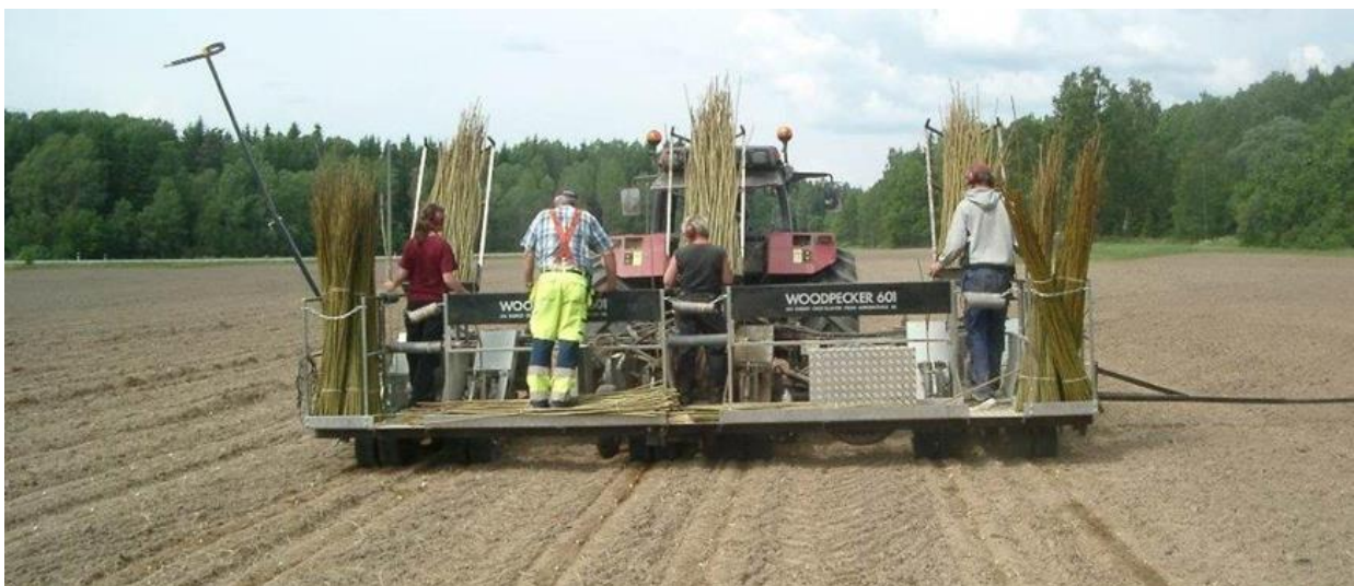
Figure 29: A willow SRC planting machine. The machine plants three double rows and needs in four persons to operate and the driver. (Source: Nordh N-E.)
