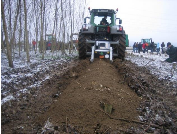
Figure 54: Cultivator for moulding the remaining SRC stumps in Austria (Source: Mergner R.)
