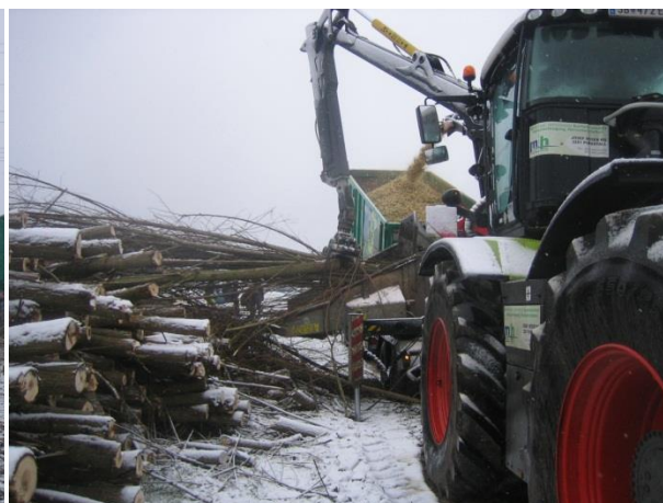
Figure 43: Woodchipper mounted on a tractor in Austria (Source: Rutz D.)
