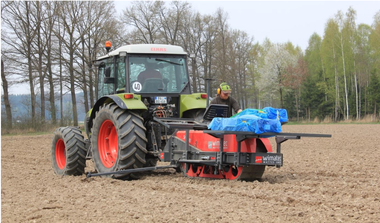
Figure 30: Planting machine for automatic planting of poplar SRC cuttings (Source: Wald 21)
