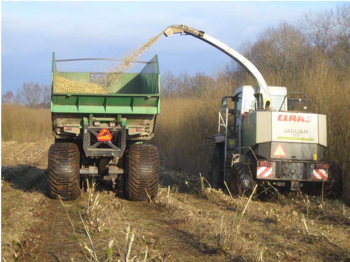
Figure 37: Claas self-propelled SRC harvester „Jaguar“ (Source: Dimitriou I.)
