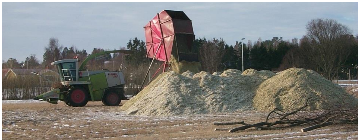
Figure 12: An SRC harvester using the broad edges of the field to temporarily store the harvested chips. The humidity of the chips will be decreased before transported to the end user. (Source: Dimitriou I.)
