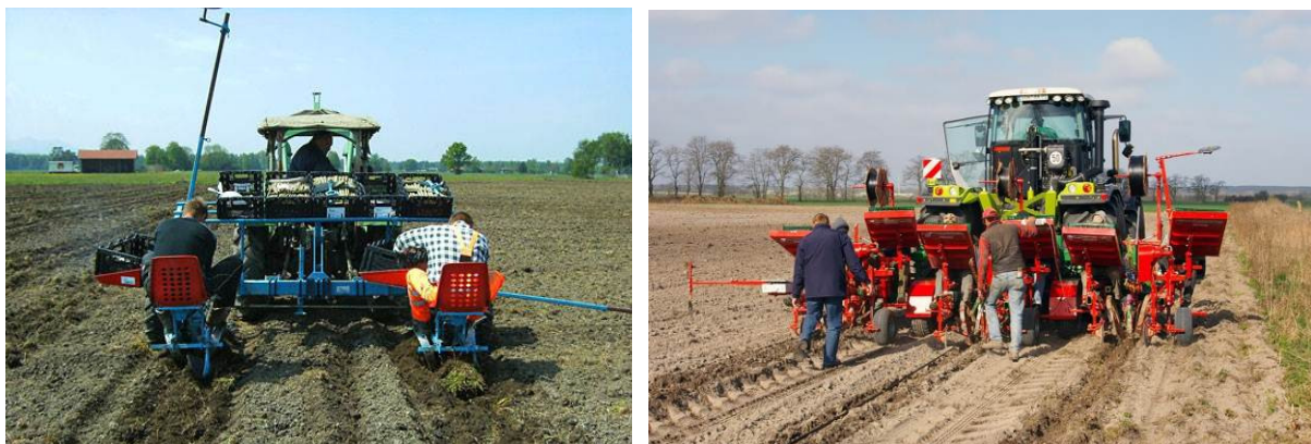
Figure 7: Tractor with the semi-automatically plantation device of Wald 21 GmbH (left, BMA 2011) and fully automatic planting machine (right, Agraligna 2011)
