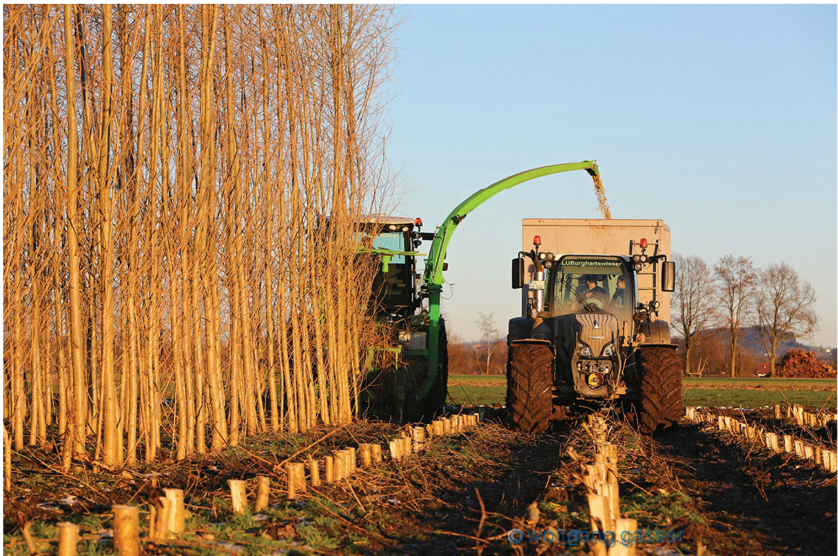
Figure 16: New harvesting prototype producing fresh SRC woodchips (2)
