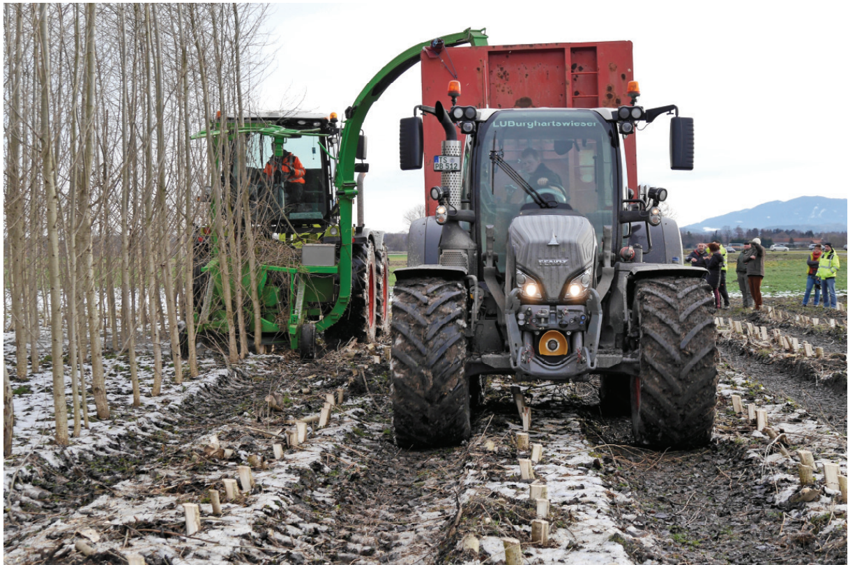
Figure 15: New harvesting prototype producing fresh SRC woodchips
