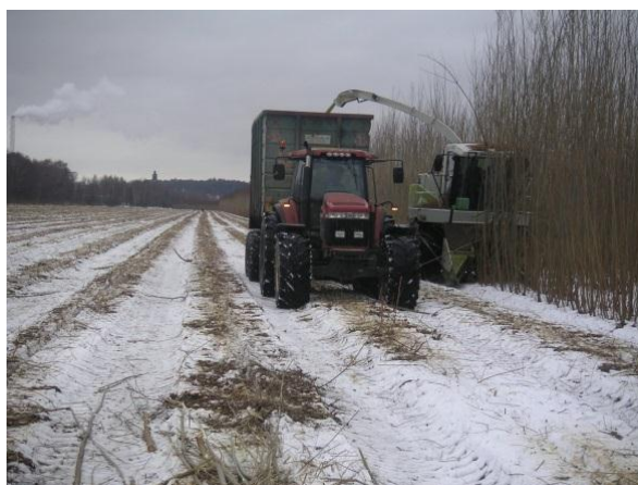
Figure 18: Winter harvest of willow SRC avoiding soil compaction, nutrient extraction from fresh parts while satisfying the peak for heating fuel needs (Photo: Ioannis Dimitriou)
