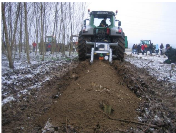
Photo 54: Broyeur de souches (Source: Mergner R.)
