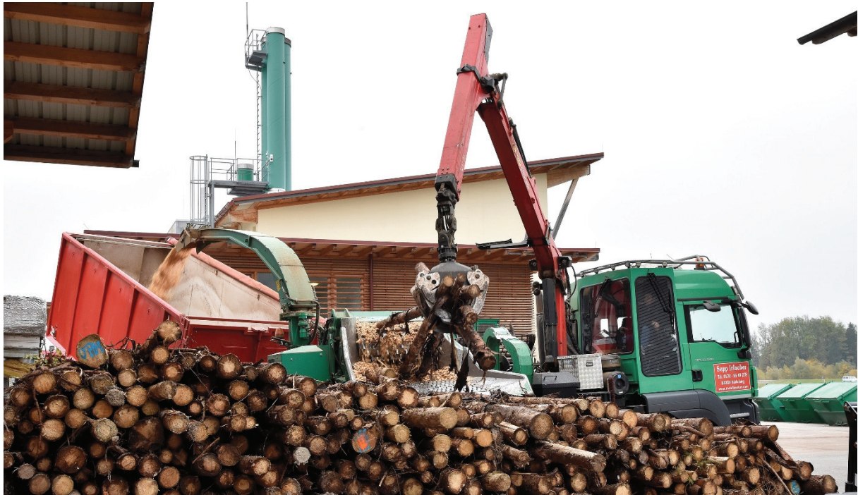
Figure 4: Real-time production of wood chips with a chipper-truck
