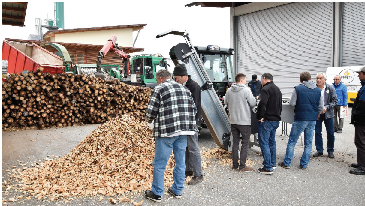
Figure 5: Real-time production of wood chips with a low-noise, smaller chipper, excellent suitable for mid- and long-term SRC trees
