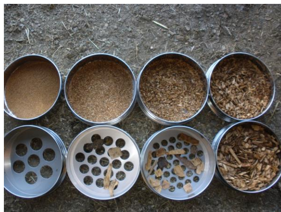
Granulometry test on SRC woodchips
